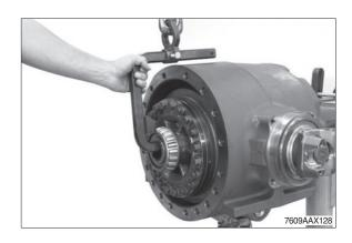
(S) Insert the determined shim (e.g. s = 1.1 mm) into the hole of the axle housing and adjust the bearing outer ring (see arrow) until contact is obtained.
