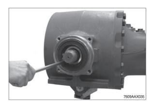
⑦ Press input pinion from the axle drive housing and remove the releasing tapered roller bearing.
