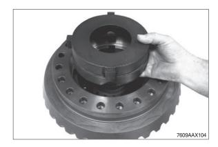
Mount outer and inner disks in alternating order, starting with an inner disk.
