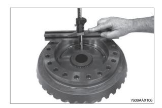
① Measure dimension II, from the contact face of the outer disk to the mounting face on the housing cover.
