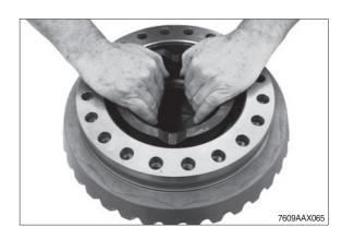
Press crown wheel from the differential carrier.
