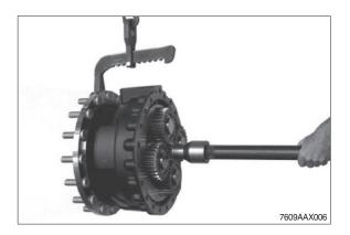
6 Fix output to assembly truck.
