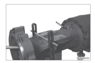
⑥ Provide screw plug with a new O-ring and fit it.
