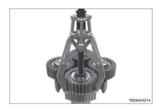
④ Lift the end plate out of the brake housing.
