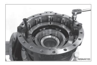
① Insert disk and cup spring with the convex side showing upwards into the piston.
