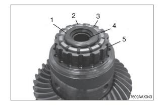
⑤ Preload differential by means of the press, loosen locking screws and housing cover.
