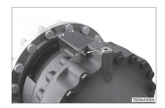
④ Secure the output with the lifting device and loosen hexagon screws.
