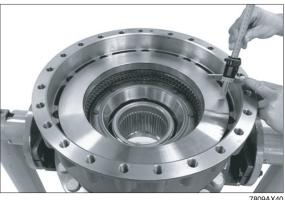
2 Press stop bolt into the cover until contact is obtained.
