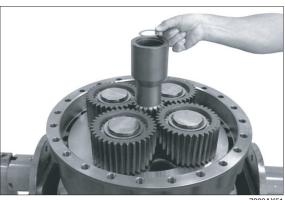
26 Fix O-ring (see arrow) with grease into the countersink of the brake housing.
