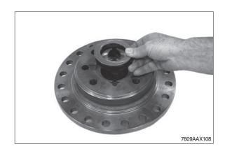
Mount two adjusting screws and insert the housing cover until contact with the differential housing is obtained.
