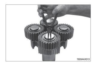
13 Pull off planetary gear.
