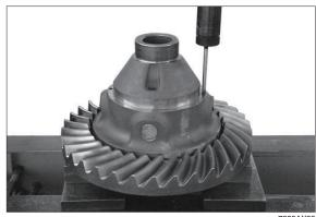
10 Pull spider shafts (4EA) and remove the releasing spider gears with the thrust washers from the differential housing.
