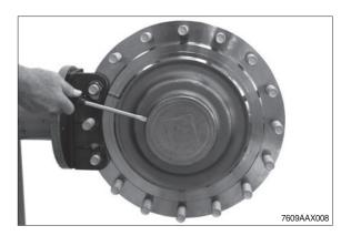
Loosen locking screws and remove the releasing cover.
