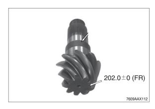
$\ensuremath{\Im}$  Determine dimension III (bearing width).
