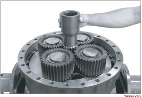
$\mathfrak{P}$  Fix determined shim e.g. s = 1.00 mmwith grease into the sun gear shaft.
