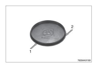
(25) Insert the cover into the output shaft until contact is obtained.
