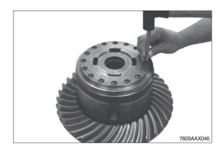
Force out both differential axles (short) and remove the releasing spider gears with thrust washers from the differential housing.
