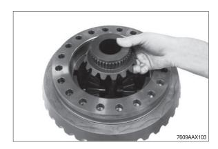
$\ensuremath{\otimes}$  Insert the second pressure ring into the differential housing.
