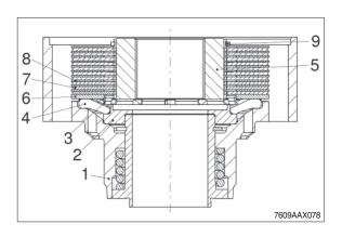
(3) Preload disk package with an axial force of  $F = 50^{+30}$  kN.
