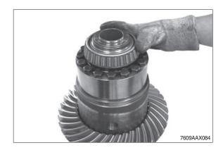
Fix axial roller cage (see arrow) to the sliding sleeve by means of grease.
