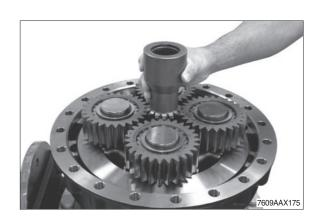
$\bigcirc$  Fix determined shim (s) e.g. s = 1.60 mm with grease into the sun gear shaft.
