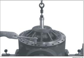
After the contact pattern check insert the differential again into the axle drive housing.
