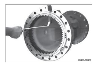
④ Pull the bearing outer ring out of the bearing hole and remove the shim behind.
