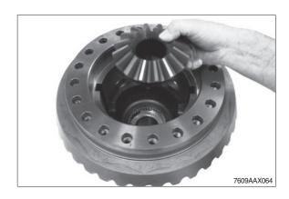
⑥ Lift the pressure ring out of the differential housing and remove the disk package and thrust washers behind.
