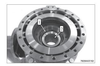
(9) Align disk package centrally and radially.
