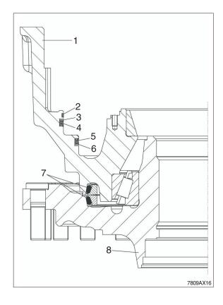
(8) Lift the brake housing from the output shaft by means of the lifting device.
