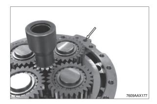
Grease O-ring (see arrow) and install it to the axle housing.
