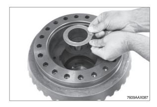
③ Insert axle bevel gear.
