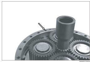
② Grease O-ring (see arrow) and install it to the axle housing.
