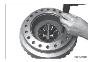
$\ensuremath{{\mbox{\scriptsize ?\!।}}}$  Mount second axle bevel gear.
