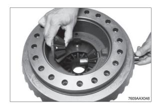
(ii) Remove the axle bevel gear and the shim behind.
