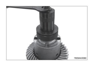
② Preload the differential by means of the press, loosen locking screws and housing cover.
