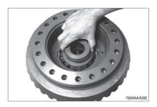
Solution 8 Fix the thrust washers into the housing cover by means of grease.
