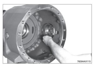
⑥ Undercool the internal bearing outer ring and bring it into contact position in the housing hole by using the assembly fixture.
