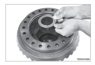
$\ensuremath{\Im}$  Insert axle bevel gear.
