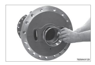
Mount two locating pins and bring the axle housing into contact position with the axle drive housing by means of the lifting device.
