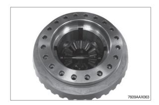
⑤ Remove the second axle bevel gear.
