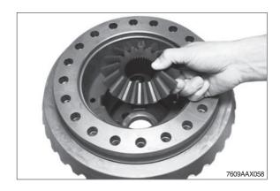
Press crown wheel from the differential carrier.
