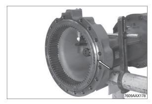
Mount two adjusting screws and use the lifting device to bring the output into contact position with the axle housing.
