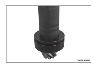
If necessary, force both bearing outer rings out of the axle drive housing.
