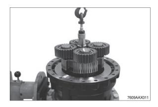
① Pull the tapered roller bearing from the planetary carrier.
