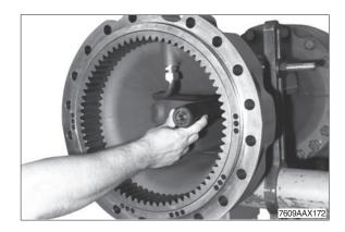
② Insert the sun gear shaft until contact is obtained.
