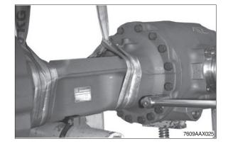
② Loosen the threaded connections and remove the releasing brake tube.
