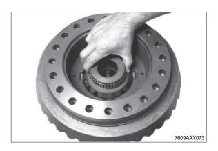
Solution 8 Fix the thrust washers into the housing cover by means of grease.
