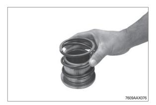
Insert the premounted sliding sleeve into the housing cover.
