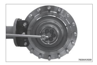
Press planetary carrier with a two-armed puller out of the profile of the output shaft.
