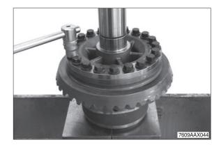
? Remove axle bevel gear with thrust washers from the differential housing.
