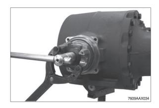
⑤ Pull the input flange from the input pinion and use a lever to remove the shaft seal behind from the axle drive housing.
