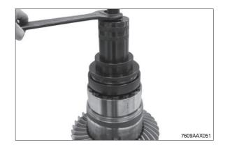
② Preload the differential by means of the press, loosen the hexagon screws and remove the releasing housing cover.
