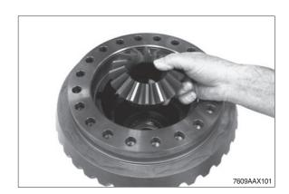
⑤ Preassemble the differential spider and insert it into the differential housing/into the pressure ring.
