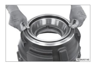
④ Insert both bearing outer rings (see arrows) into the brake housing until contact is obtained.
