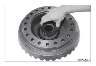
$\ensuremath{\mbox{\Large 5}}$  Force out both slotted pins.
