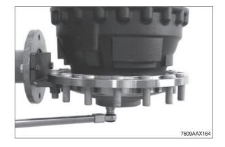
② Pivot output 180° and measure gap width from the output shaft to the planetary carrier (see also subsequent sketch).
