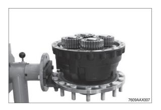
① Use a lever to remove the cover from the output shaft.
