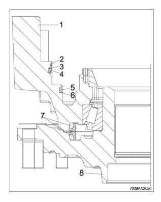
(1) Lift the brake housing from the output shaft by means of the lifting device.
