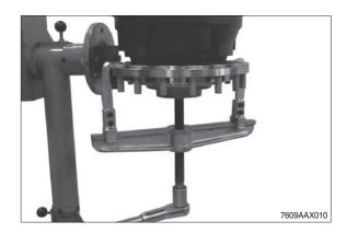
① Lift the planetary carrier out of the brake housing by means of the lifting device.
