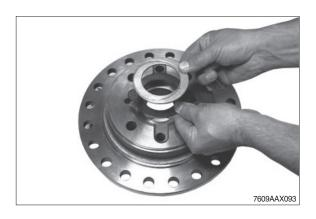
Mount two adjusting screws and insert the housing cover until contact with the differential housing is obtained.
