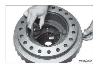
Remove the axle bevel gear and the shim behind.
