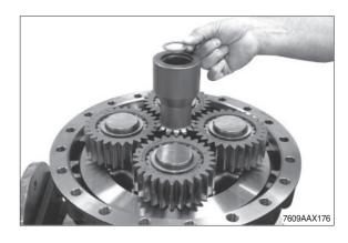
② Fix O-ring (see arrow) with grease into the countersink of the brake housing.
