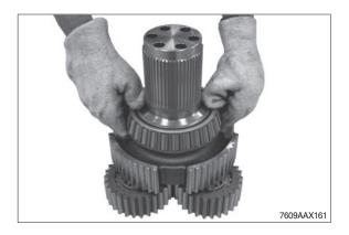
Wet front face (contact face bearing inner ring, arrow 1) and profile (teeth, arrow 2) in the output shaft with anticorrosive agent.
