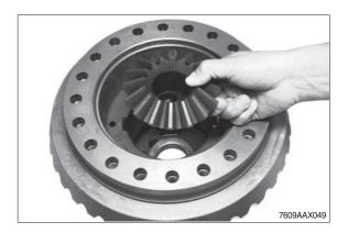
Press crown wheel from the differential carrier.
