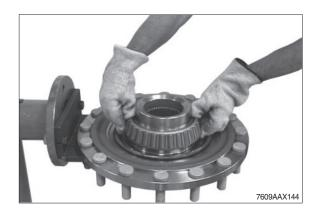
Wet O-ring of slide ring seal and locating hole with spirit.
