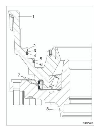
6 Insert the piston into the brake housing and carefully install with the fixing device until contact is obtained.
