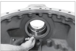
3 Undercool the internal bearing outer ring and bring it into contact position in the housing hole by using the assembly fixture.
