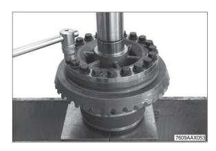
④ Remove axle bevel gear with thrust washers from the differential housing.
