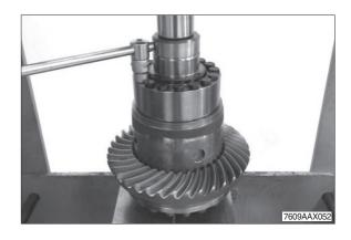
③ Preload the differential by means of the press, loosen locking screws and housing cover.
