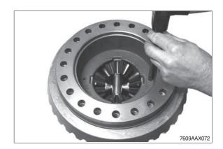
$\ensuremath{{\bigcirc}}$  Mount second axle bevel gear.
